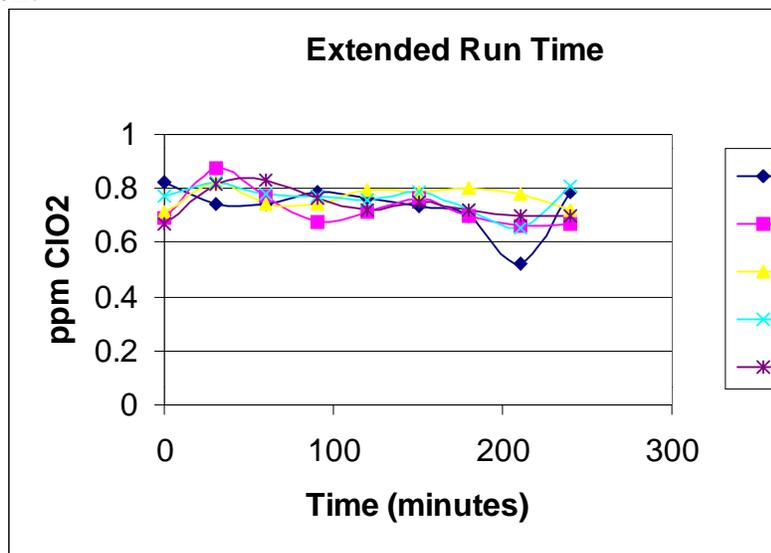
maintained a reasonably stable output over the four hour test period.
