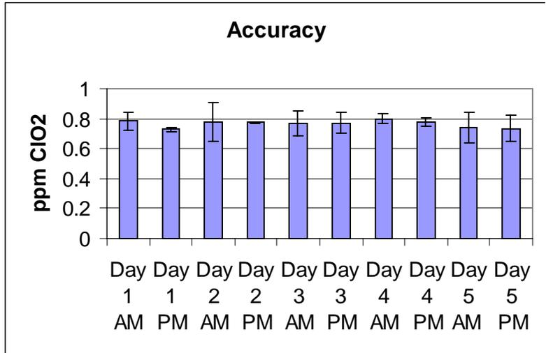
Although the generator was set to produce 1.00 ppm chlorine dioxide, the average measured concentrations consistently fell between 0.72 ppm and 0.80 ppm throughout the week. The coefficient of variation for chlorine dioxide output over the course of the week was 7.54%.
