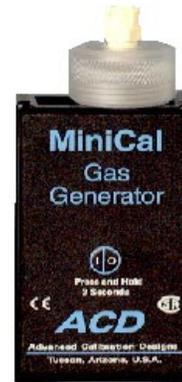
The MiniCal is a small, battery-powered, portable electrochemical gas generator designed to calibrate toxic gas sensors. Fast warm-up time allows the instrument to be turned off between remotely located sensors saving battery life and avoiding generation of unwanted gas. The MiniCal uses the following components to produce the calibration gas/air mixture:
