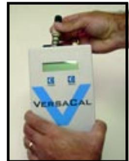
Before inserting into the instrument, firmly squeeze the QCV so that the inner ampoule is broken. Install the QCV onto the end of the QCV holder. Place the QCV and the QCV holder in the vial chamber, pushing it in firmly until the o-ring makes a complete seal.
